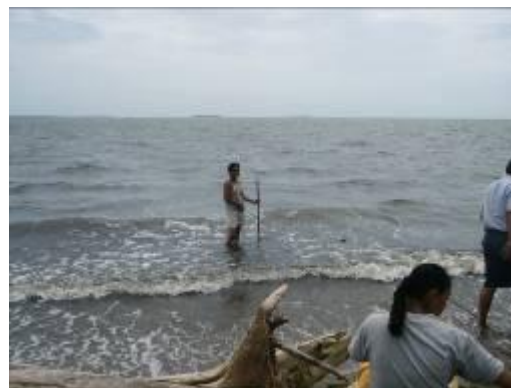
Measuring wave height with a wave pole in Fiji
